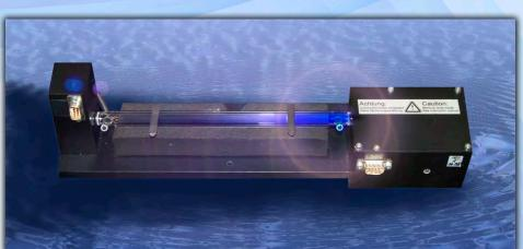
controlled by a reference beam and reference detector device. In addition to this, the UV detectors of the UT-3000 are thermostatically controlled. Heating of the optical cell and the GoldTrap makes the UT-3000 insensitive to volatiles like water vapor and hydrocarbons.
